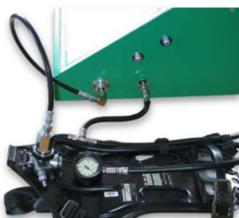
SCBA connected to a Multicheck eco VX3 for testing
