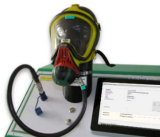
SCBA connected to a Multicheck eco VX3 for testing
