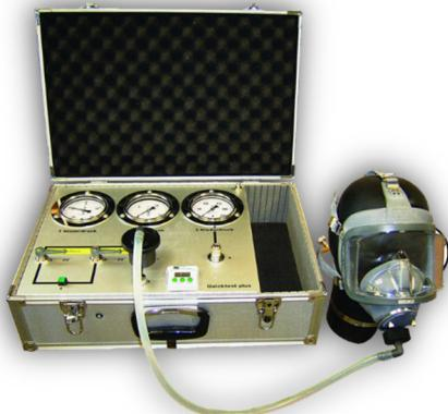
Quicktest plus can be used for performing static as well as dynamic tests on diving gear and, with an optional upgrade, buoyancy compensator devices (BCD). In this context, it is important to keep in mind that connectors and the scope of required functional tests may vary from one make of diving equipment to another.
