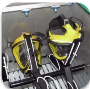
Masks fastened to the rotating mask holder by means of elastic straps
