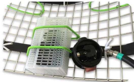
Flexible elastic straps keep the LGDVs securely in place
